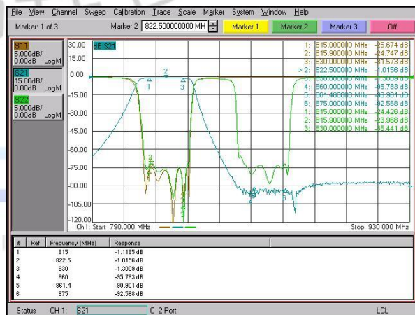
Duplexer UL path Transmission
